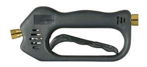
The linear high pressure spray gun ST-601, can be used for professional high pressure cleaning with hot and cold water. The handle housing is made of impactresistant plastic. The valve housing and the connections are made of corrosion-resistant material. The trigger is equipped with a safety catch.
