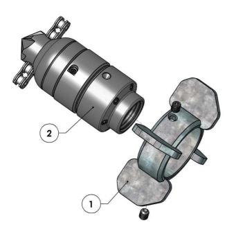
Short centralizers for Avian nozzles are advisable when using the nozzle with the chain head. Insert the nozzle (2) in the leading ring (1) from the side where the blocking screws are closer to the nozzle edge. Tighten the two locking screws using a straight hexagon 2,5 mm screwdriver. Check regularly that the two dowels are not loosened, eventually tighten them using a thread locker like Loctite 243.
