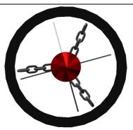
Figure 2: Nozzle with centralizer, properly placed
